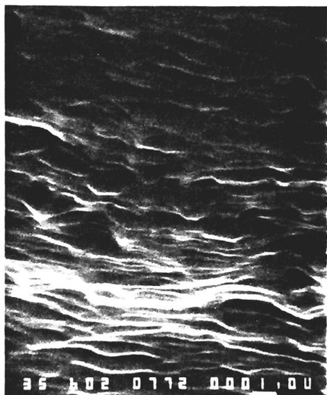
**FIG. 5.** The tearing topography surface of the  $\Sigma 11$  bicrystal. (723 K in vacuum for 96 hours)
