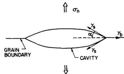
Fig. 6. Geometry of double spherical cap-shaped nucleus.
