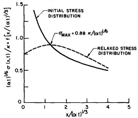
Fig. 3. Initial and relaxed stress distribution plotted using normalized coordinates suggested by the analysis.
