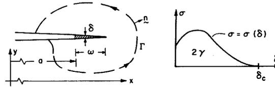
Fig. 4. Cohesive zone model for elastic-brittle fracture. Path  $\Gamma$  for evaluation of  $J$  integral may be shrunk to boundary of cohesive zone, showing equivalence of cohesive zone model and Griffith criterion when  $\omega$  is small compared to overall geometric dimensions.
