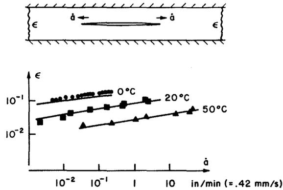
Fig. 9. Data of Mueller and Knauss on crack growth in Solithane 50/50; solid lines from analysis by Schapery based on cohesive zone model.
