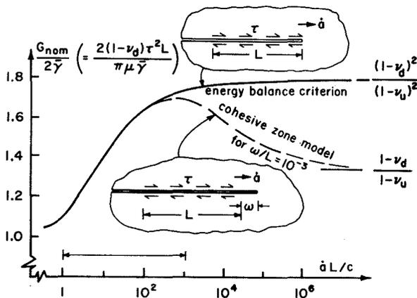
Fig. 10. Shear crack growth in a fluid-infiltrated elastic solid. Comparison of energy balance criterion with cohesive zone model. Curves are drawn for  $(1-\nu_d)/(1-\nu_u) = 1.33$ . Marked portion of speed axis corresponds to range of observed fault creep events; see text.
