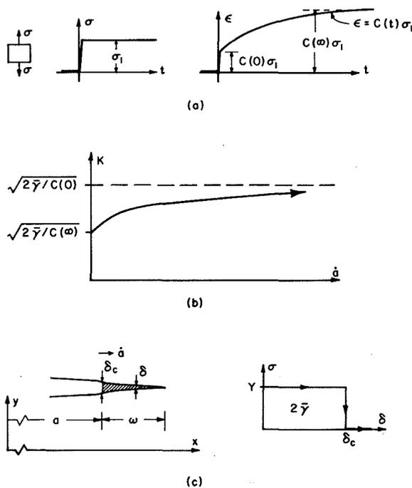
Fig. 8. Crack growth in linear viscoelastic solid. (a) Definition of creep compliance function  $C(t)$  for plane-strain tension test. (b) Expected form of relation between stress intensity factor and crack growth rate. (c) Cohesive zone fracture model.
