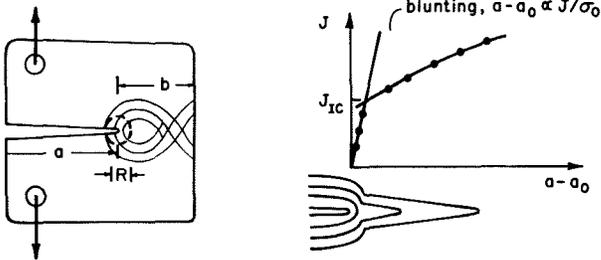
Fig. 12. Early stages of ductile crack growth and definition of  $J_{IC}$ .  $R$  denotes zone dominated by the  $J$ -characterized singularity at crack tip. See text for discussion of conditions under which the  $J$  versus  $a-a_0$  relation may be considered as a "resistance curve," characteristic of the material.
