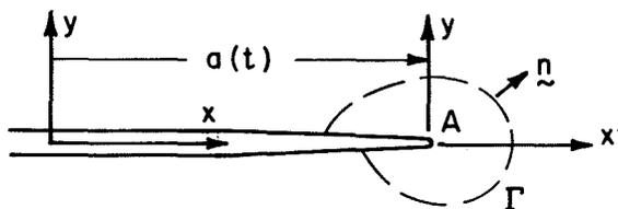
Fig. 7. Notation for discussing energy flux to a mathematically sharp, structureless crack tip; the  $x'$ ,  $y$  axes, region  $A$ , and contour  $\Gamma$  move through the material with the tip.
