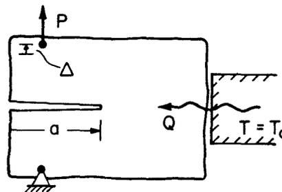
Fig. 3. Griffith crack in body at temperature T<sub>0</sub>; for discussion of thermodynamic restrictions on crack growth.
