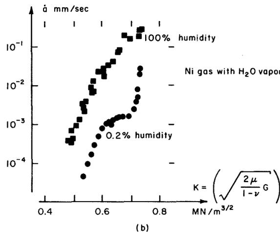
Fig. 6. Data of Wiederhorn on time-dependent crack growth in glass. (a) 61% lead glass in vacuum. (b) Soda-lime-silica glass in environments of nitrogen gas with water vapor.
