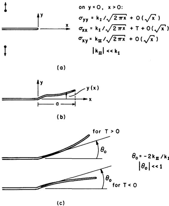
Fig. 2. Stability of the straight path of crack growth under mode I (tensile) loading. (a) Stress field near tip of crack loaded in tension; imperfection of loading system results in small mode II stress intensity. (b) Notation for describing extension of crack. (c) Crack path is unstable if  $T > 0$ , based on growth condition that  $K_{II} = 0$  at advancing crack tip.
