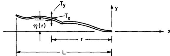
Fig. 1. Slightly curved or kinked two-dimensional crack. Coordinates are oriented so that x-axis is tangent to the crack at its tip;  $T_x$  and  $T_y$  are the surface tractions.
