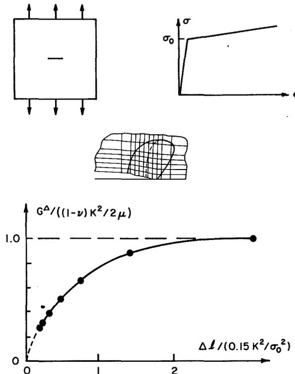
Fig. 11. Elastic-plastic finite-element results of Kfourri for energy release rate based on finite crack growth steps (equal to element size,  $\Delta l$ ). Growth step is normalized by approximate measure of the maximum extent of plastic zone, and results seem consistent with theoretical result that  $G=0$  for continuously growing crack.
