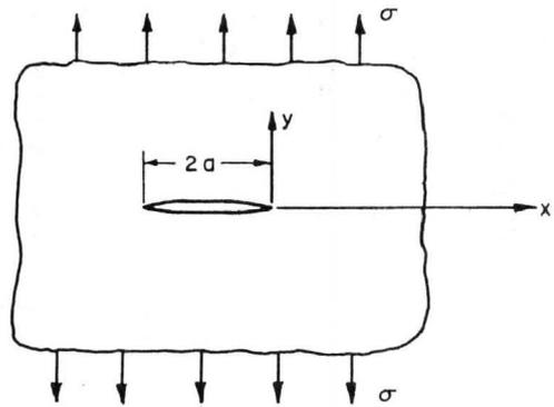
FIG. 8 FINITE CRACK IN TENSILE FIELD
